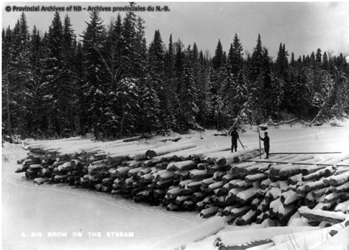
Logs piled on stream in preparation for spring thaw and subsequent log drive.
